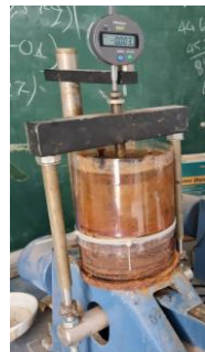
Figure 2.13: Modified oedometer apparatus for side friction pressure measurement
